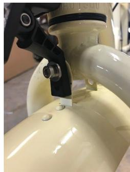
**Front wheel and brake disc placement in center of disc caliper**
